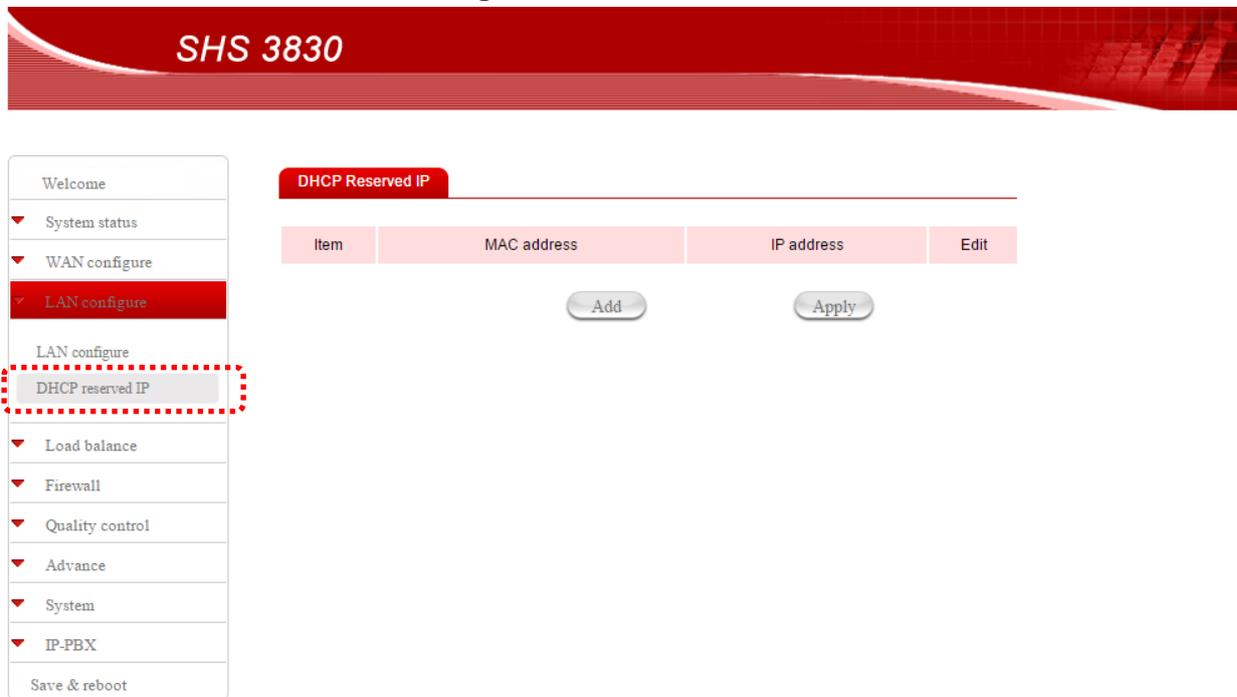
Step 2: Fill data to MAC address and IP. Then Click “Add” then SHS 3830 goes back to **DHCP reversed IP** list table. The input screen shows as follows.
